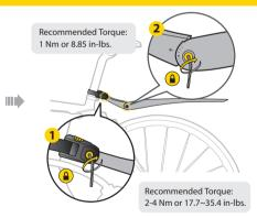
Adjust DeFender™ iGlow for proper angle and tire clearance. Retighten the adjusting bolts once the correct angle is achieved.
